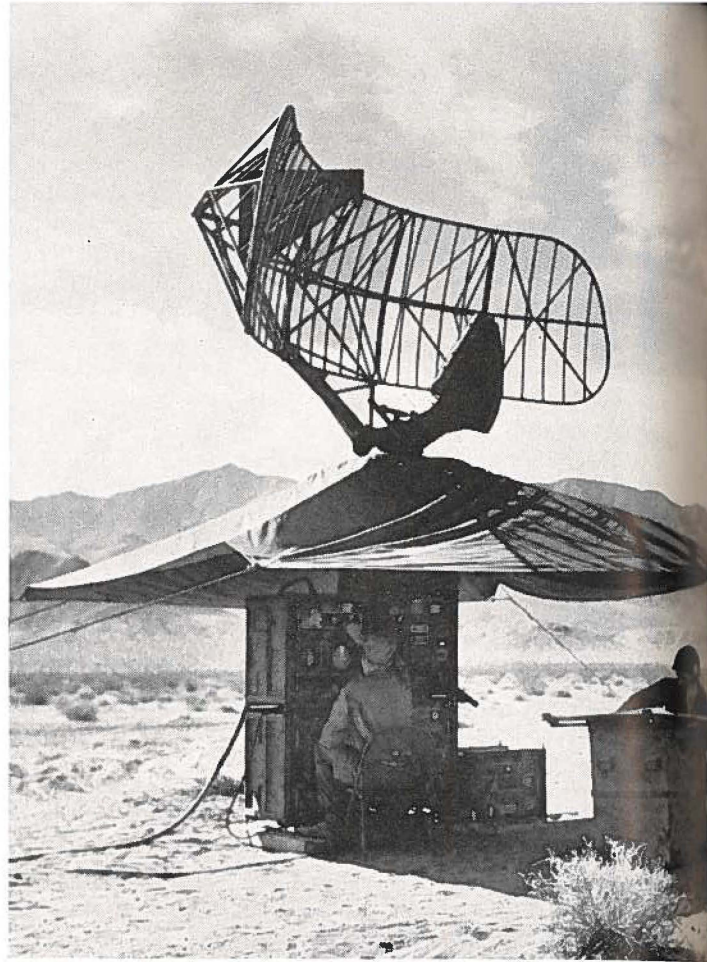
Men of the 746th AAA Bn California National Guard manipulate the controls of their AN/TPS-1D radar surveillance unit during summer training at Camp Irwin, California. The data from their "Topsy Dog", as the troops call this particular radar set, is piped to the central operations van. —U. S. Army Photo
