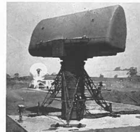
ACQUISITION radar picks up approaching aircraft. White ball (left background) is missile tracking radar.
