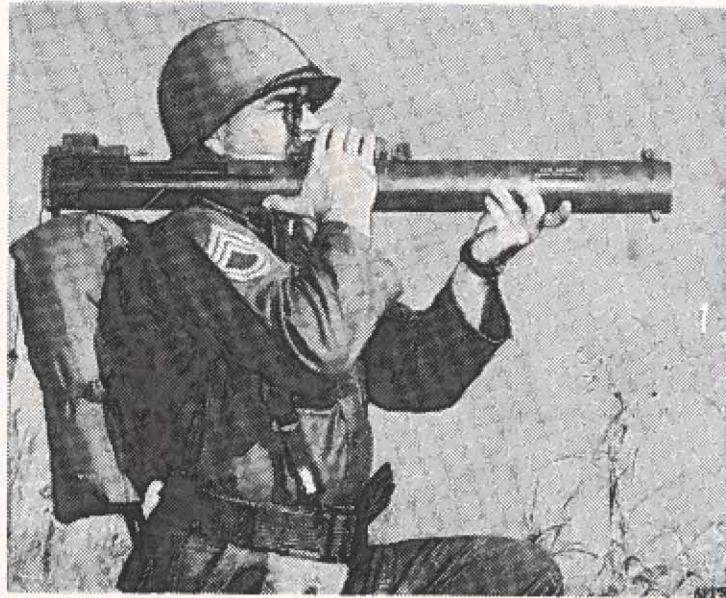
DISPOSABLE WEAPON —This new Army anti-tank weapon, the XM72 rocket grenade, comes packed in an aluminum lined, fiberglass-plastic tube that serves as its launcher and can be thrown away after firing. Weighing only four and a half pounds, the weapon can be fired kneeling as shown or from the standing or prone positions. The rocket's solid-propellant projectile is effective against tanks, armored vehicles and field fortifications.
