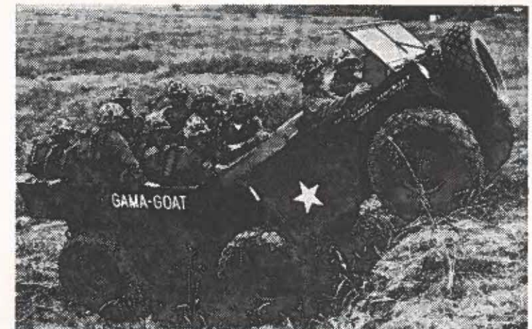
BROKEN FIELD RUNNER —Chance Vought Corporation's "Gama Goat" is the newest entry into the field of mobile military vehicles. An 80 hp., air-cooled engine drives this six-wheeled amphibious vehicle which can travel over rough terrain or across rivers with a heavy load of personnel, armament or equipment.
