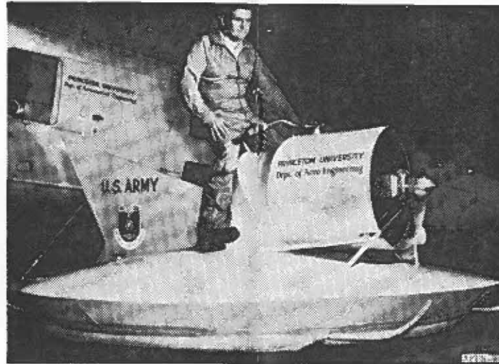
FLYING SCOOTER —Helicopter mechanic Bart Reavis drives the flying scooter that rides on a cushion of air and handles like a bicycle. The scooter was developed by Princeton University under a grant provided by the Army. The driver's only controls are a pair of handlebars and a sense of balance.
