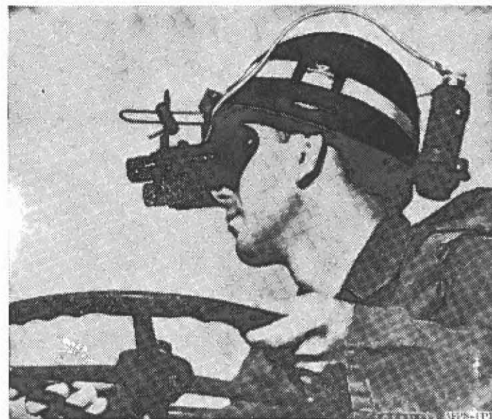
NOCTURNAL VISION —Darkness, like rough terrain, is no obstacle to the mechanical mule when the driver is equipped with infrared binoculars. Developed by the Army Corps of Engineers at Ft. Belvoir, Va., the binoculars also make construction in total darkness possible.
