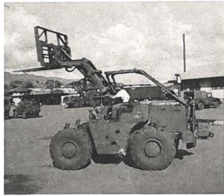
One of the most versatile pieces of new Guard equipment is the rough terrain forklift, being used at each of the NIKE sites. The gasoline-driven lift weighs 15 tons and can lift a five-ton load.
