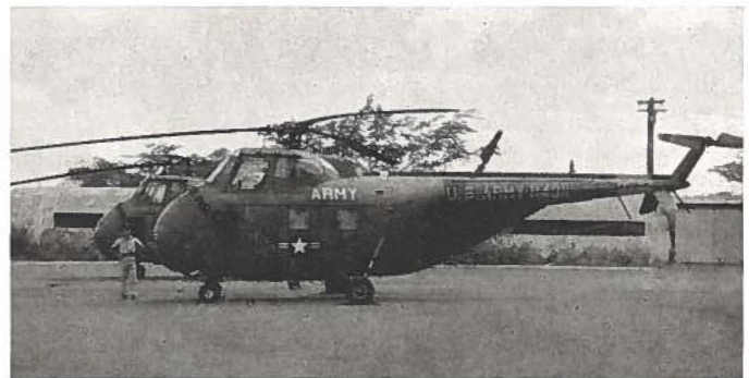
These two H-19 utility-type helicopters are now in HARNG inventory and are being flown by the aviation section. Capable of carrying 10 passengers and a crew of three, the 'choppers cost $137,000 each. In addition to these rotary-wing aircraft, the Guard operates two H-13 Bell helicopters.
