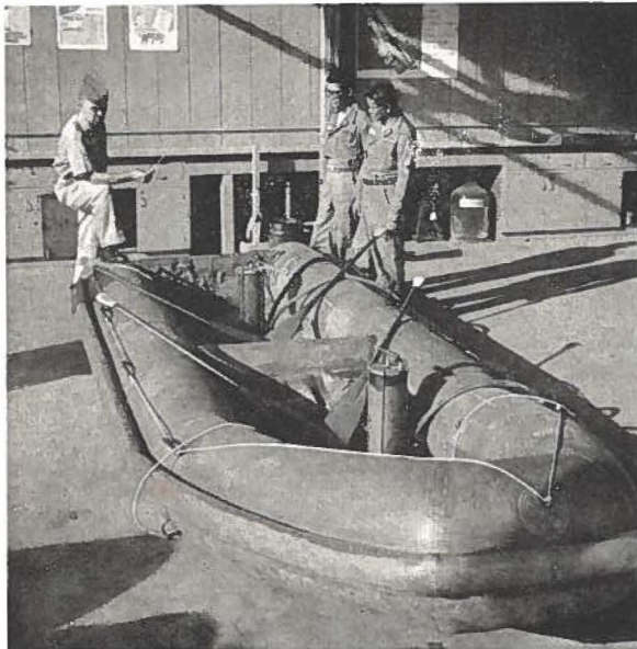
The 227th Engr Bn has 18 of these rubber river assault boats and is the only Guard unit in the U.S. to have them. The $790.00 boat holds 15 men and may be modified for use as floating bridge type raft.
