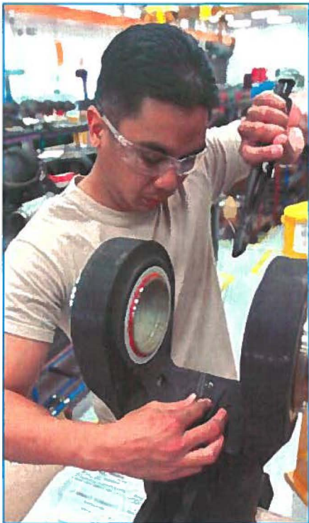
Spc. Willie Fetu, a UH-60 Black Hawk helicopter repair technician, attaches safety wire to a Black Hawk's main rotor assembly.
