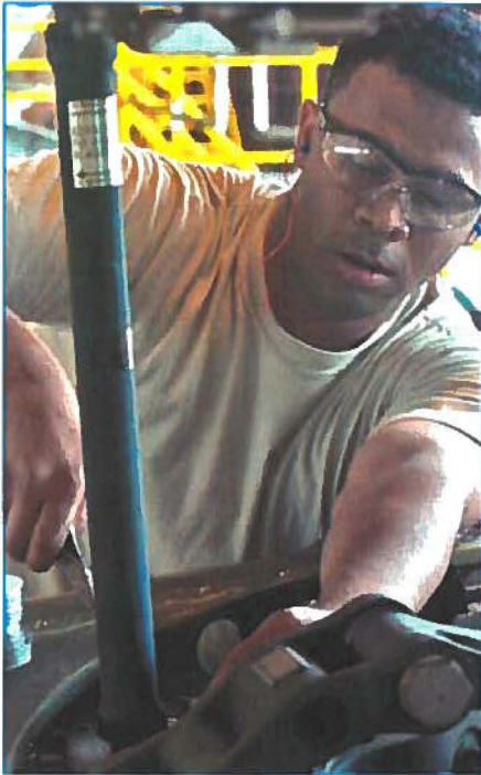
Staff Sgt Jarrett Cummings, an aircraft power train repair technician, attaches a safety wire to the main rotor head-unit of a UH-60 Black Hawk.
