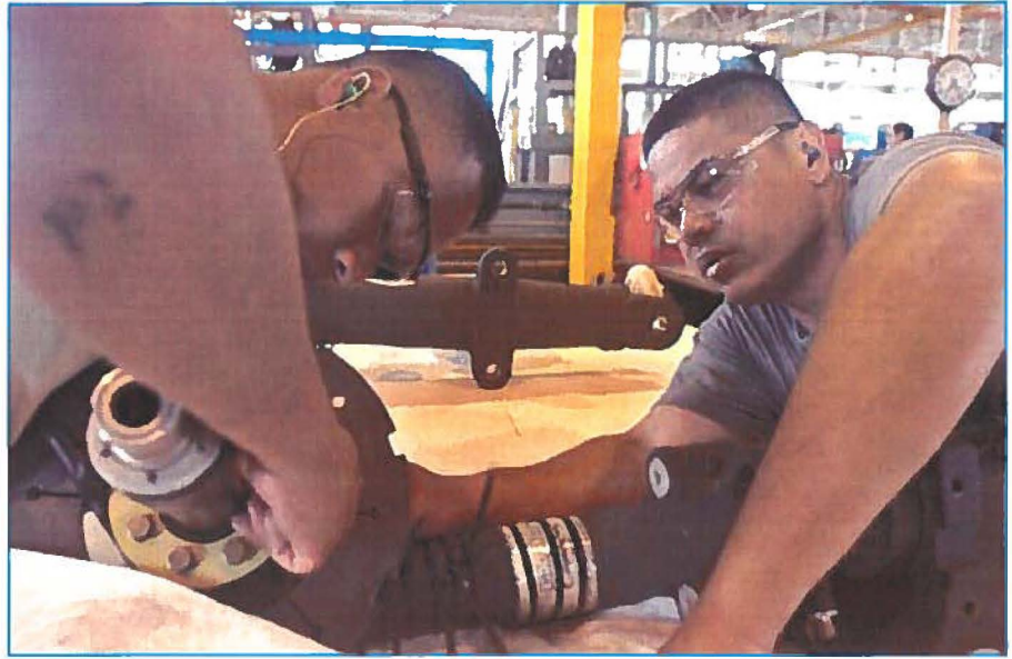
Spc. Phuc Huyhn and Sgt. Ignacio Boroga, CH-47 Chinook helicopter repair technicians, secure a brake pad to a Chinook's landing gear.
