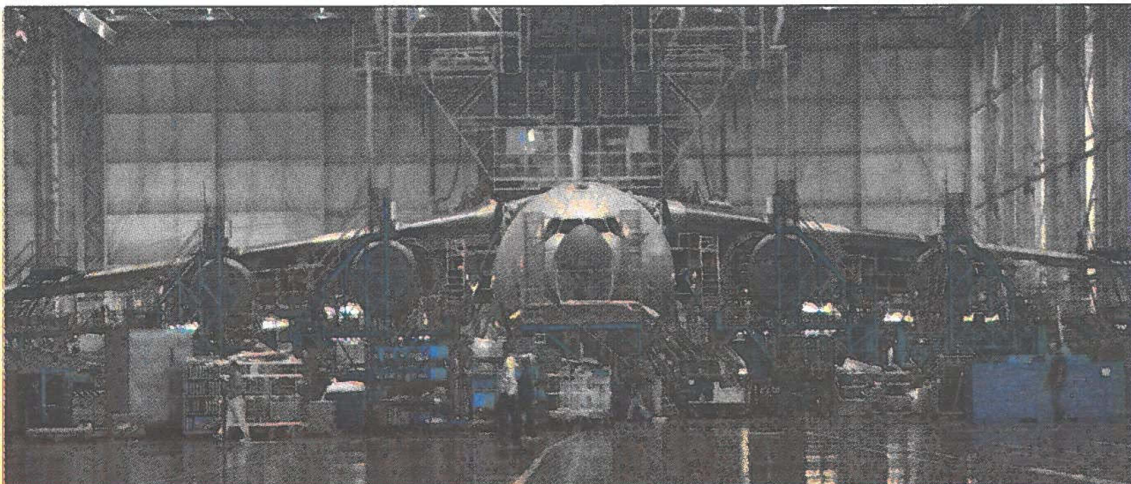
The first C-17 scheduled to arrive at Hickam AFB in early February, begins to take shape after a major join ceremony Aug. 19, at the Boeing facility in Long Beach, Calif. The ceremony, in which the wings are attached to the body of the aircraft, is the first time the C-17 looks like its finished product. Photo by Tech. Sgt. Kristen Higgins
