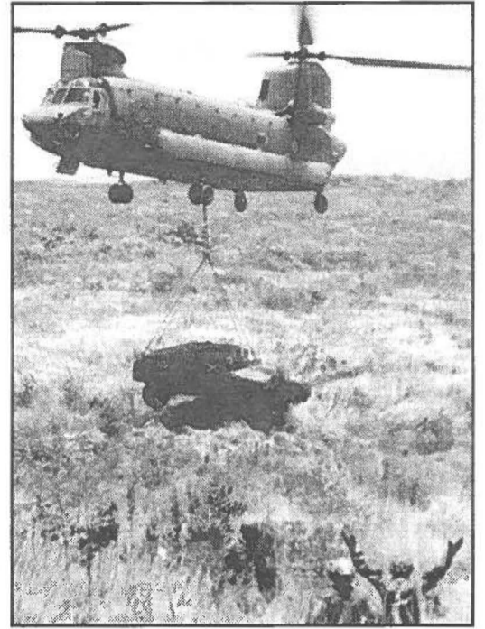
Maj. R. Scott Rhode RECOVERY MISSION — A CH-47D Chinook helicopter from Co. C (Medium Lift), 193rd Aviation, airlifts a 29th Separate Infantry Brigade hummer to the Pohakuloa Training Area motor pool.
