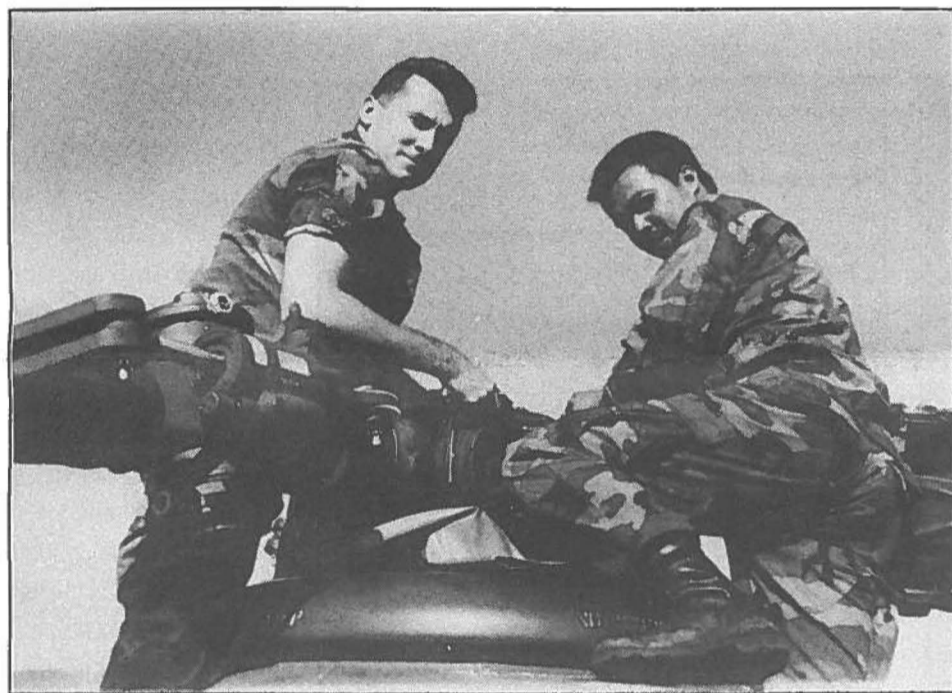
ROTARY WINGS —Sgt. Michael Pray (L), and Spc. Warnee Bagay, Aircraft Mechanics of HIARNG's B Co. 1/1 93 perform end-of-phase maintenance checks on a CH-47 of the U.S. Army's 25th Infantry Division.
