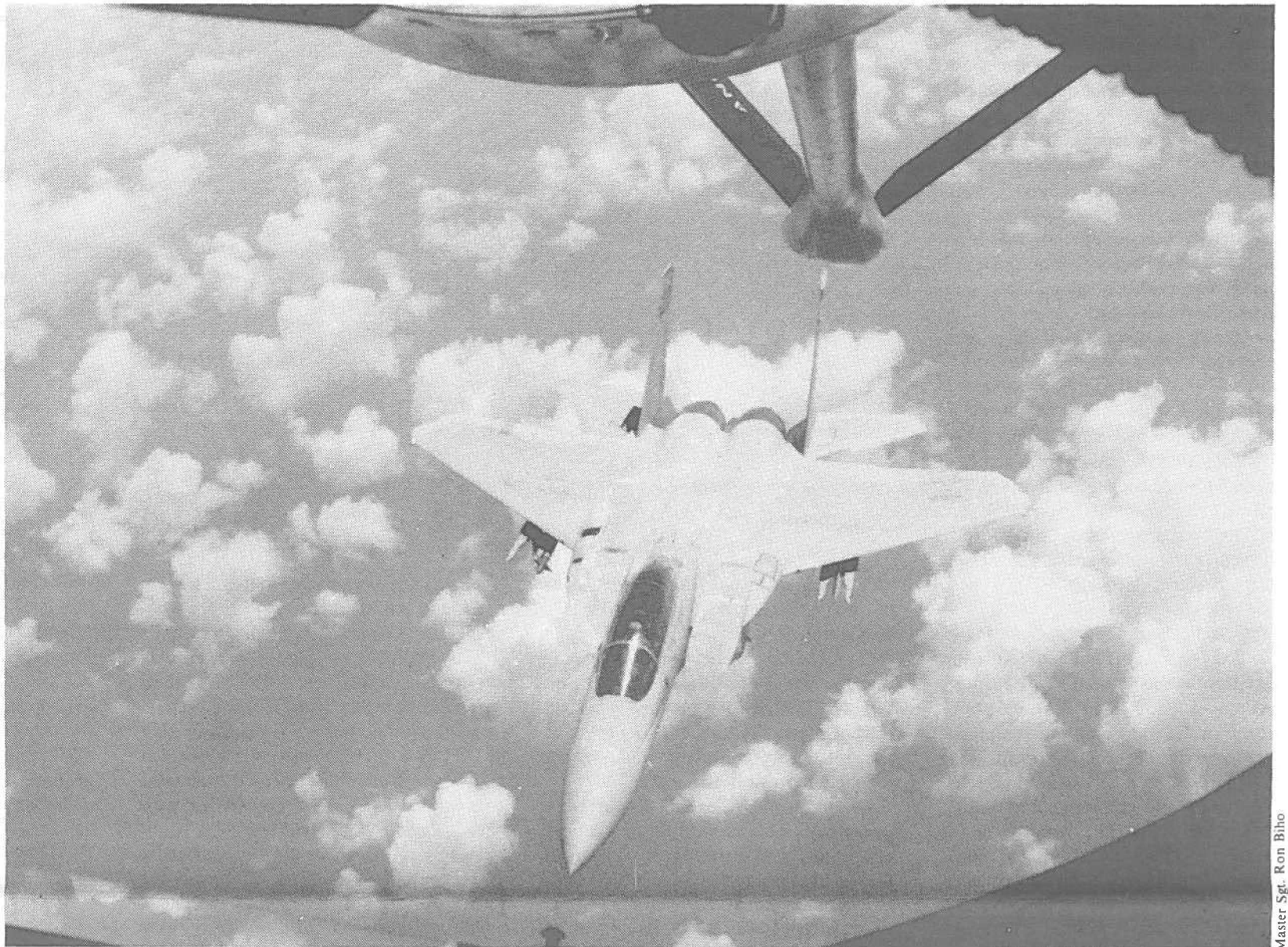
FILL-IT-UP —An F-15 Eagle from the Hawaii Air National Guard is refueled from an Arizona Air National Guard KC-135 Stratotanker during Sentry Tigre.
