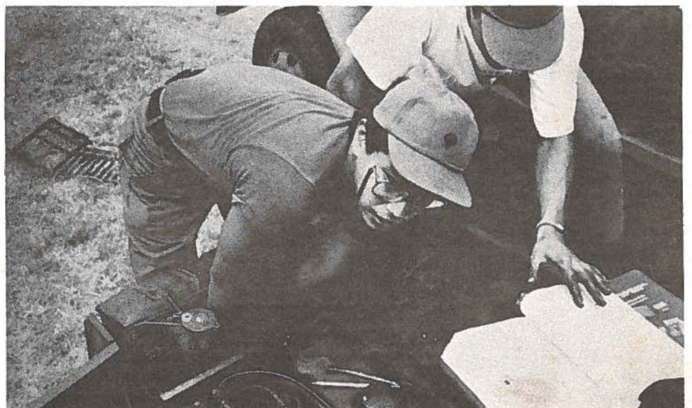
WHAT DO I DO NEXT? — Sp4 Gerado Pascua, left, and Pvt. Darryl Akana use "the book" while replacing a water pump on a 2 1/2 ton truck at Area X. — Photo by Sp5 John Atkinson.
