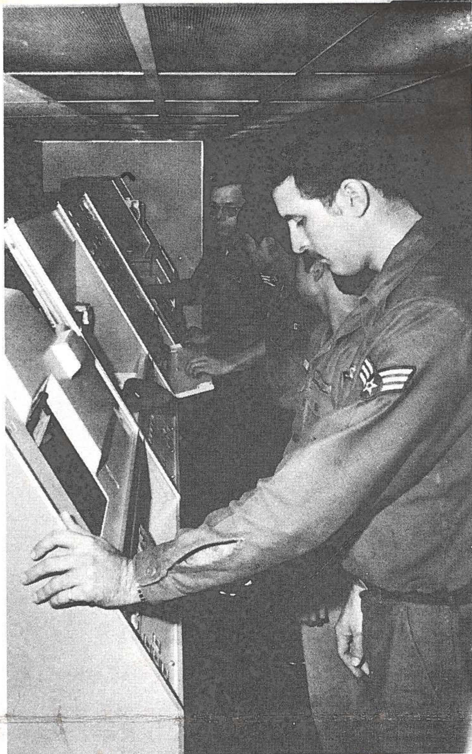
The on-line van includes (front to rear) a card reader, dual tape reader, control console, card punch, printer and tape punch.
