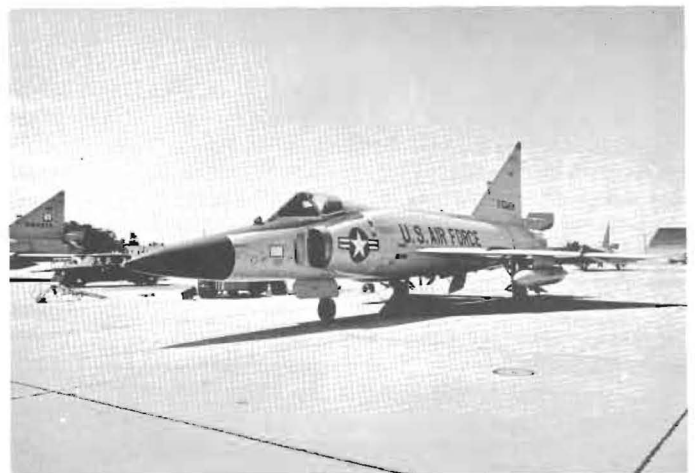
THE LATEST MODIFICATION to the Hawaii Air National Guard's F102s was the installation of wing tanks to give the interceptors greater range. The tanks can be dropped in case of emergency.
