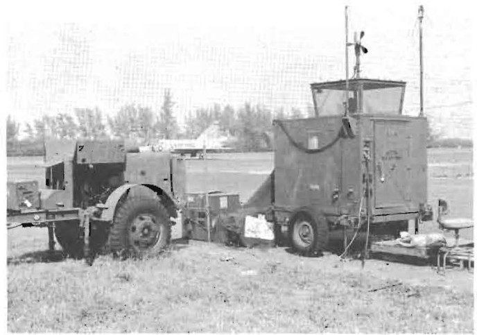
AN UNIDENTIFIED MEMBER of the 201st Mobile Communications Squadron directs an F102 flown by the 199th Fighter Interceptor Squadron, HANG, to a safe landing using a portable control tower. This same type of tower was deployed to the Kona Airport by the 201st Mobile Communications Squadron in a joint project with the FAA.
