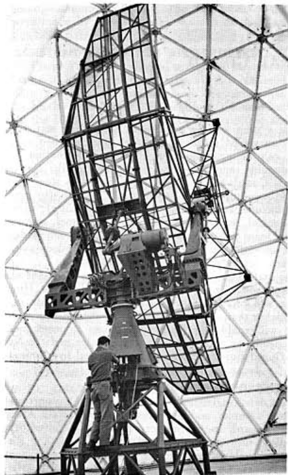
Radar antenna inside huge white plastic dome is one of two types located atop Mount Kaala, Oahu. This station is soon to be manned by Air Guard and FAA personnel. Plastic dome is 50-feet in diameter; can withstand winds in excess of 150 mph.
