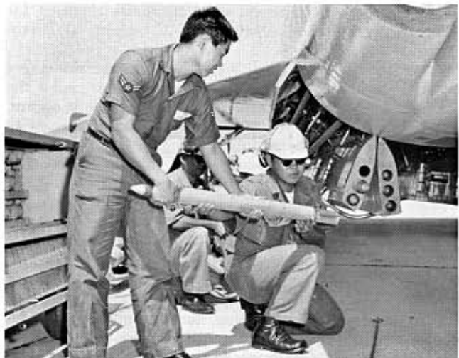
Air Guardsmen load rockets into belly of supersonic F-102 fighter. Jet carries 24 folding-fin rockets and six guided missiles.
