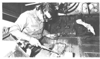
MSgt. Joseph Viveros repairs the flooring of 1/4 ton jeep.
