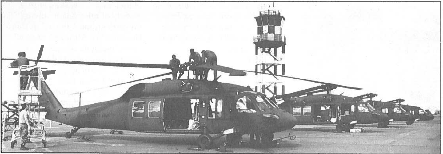
BLADE RUNNERS -- Hawaii and California Army National Guard aviation mechanics assemble UH-60 Blackhawk helicopter blades at Hickam Air Force Base, July 19, 1994.
