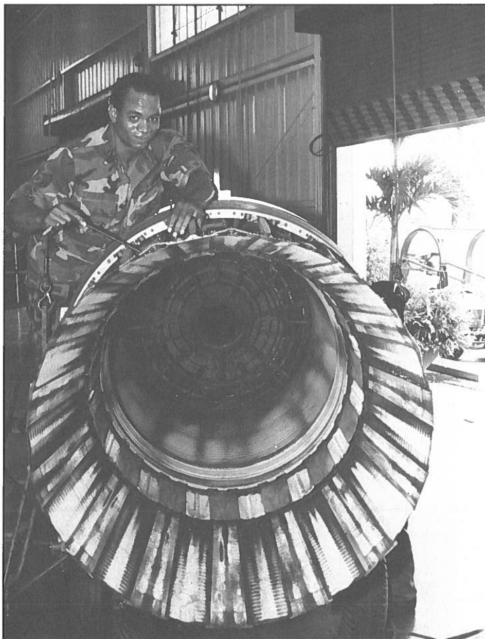
POWER CHECK -- An airman from the the Hawaii Air National Guard's 154th Consolidated Aircraft Maintenance Squadron checks an F-15 aircraft engine at the squadron's Hickam Air Force Base engine shop.
