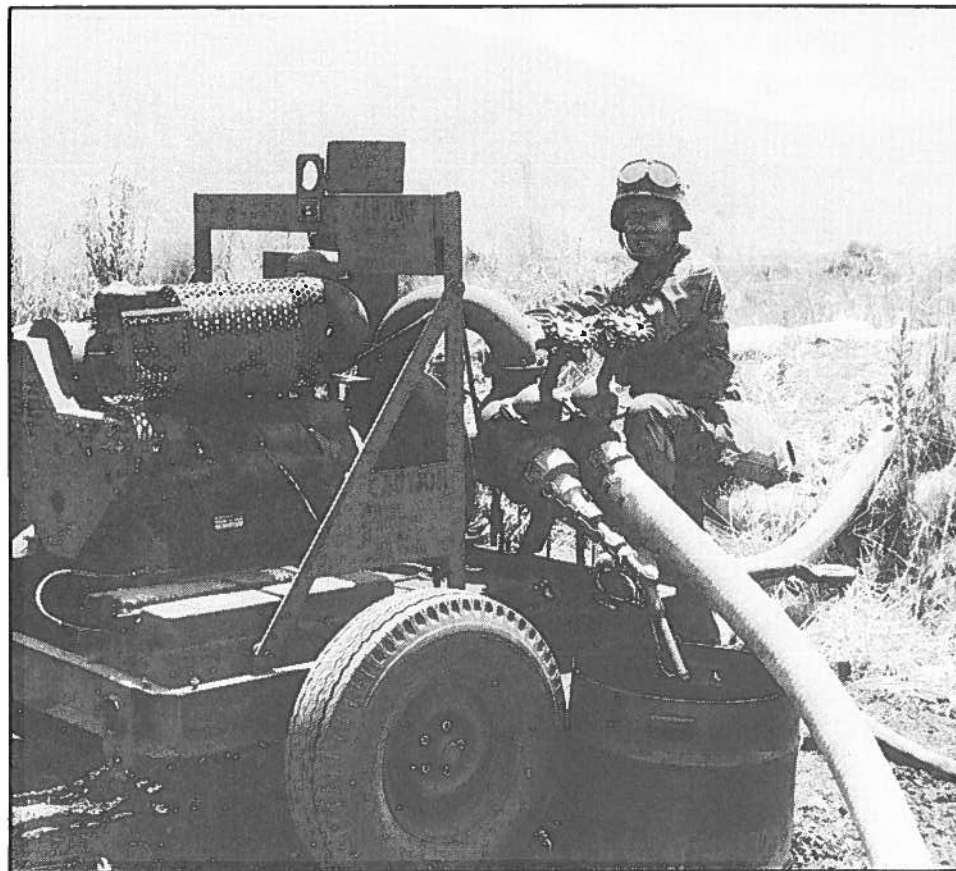
A 292nd Service and Supply Company soldier uses a generator pump unit to transfer fuel from a truck to a 10,000-gallon bladder (rubber storage bag) at the Pohakuloa Training Area on the island of Hawaii.
