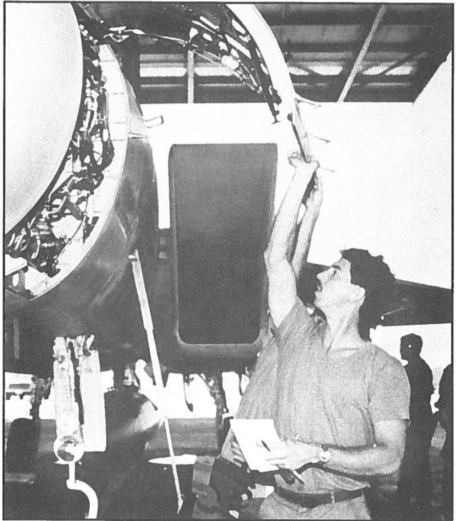
An airman from the 154th Consolidated Aircraft Maintenance Squadron checks the F-15 Eagle's electronic compartment prior to takeoff.
