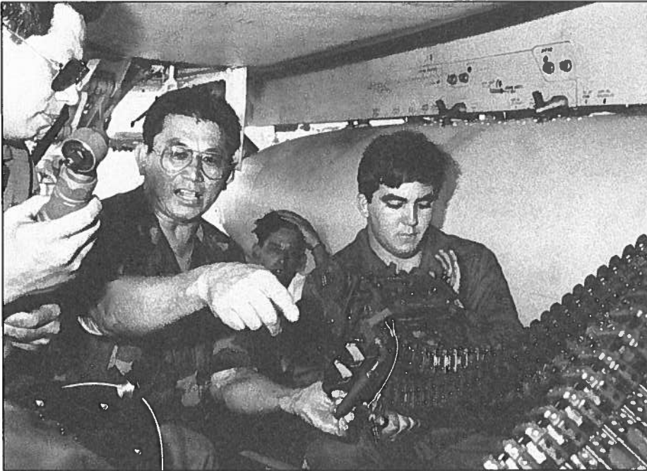
Aircraft maintenance airmen learn how to load 20mm MO1A1 munitions into the F-15's gatling gun.
