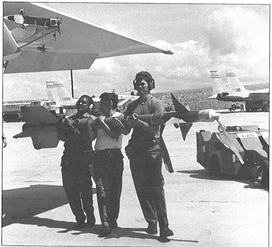
A 154th Consolidated Maintenance Squadron load crew prepares to mount an AIM 9L sidewinder air-to-air missile onto the wing of an F-15 Eagle.
