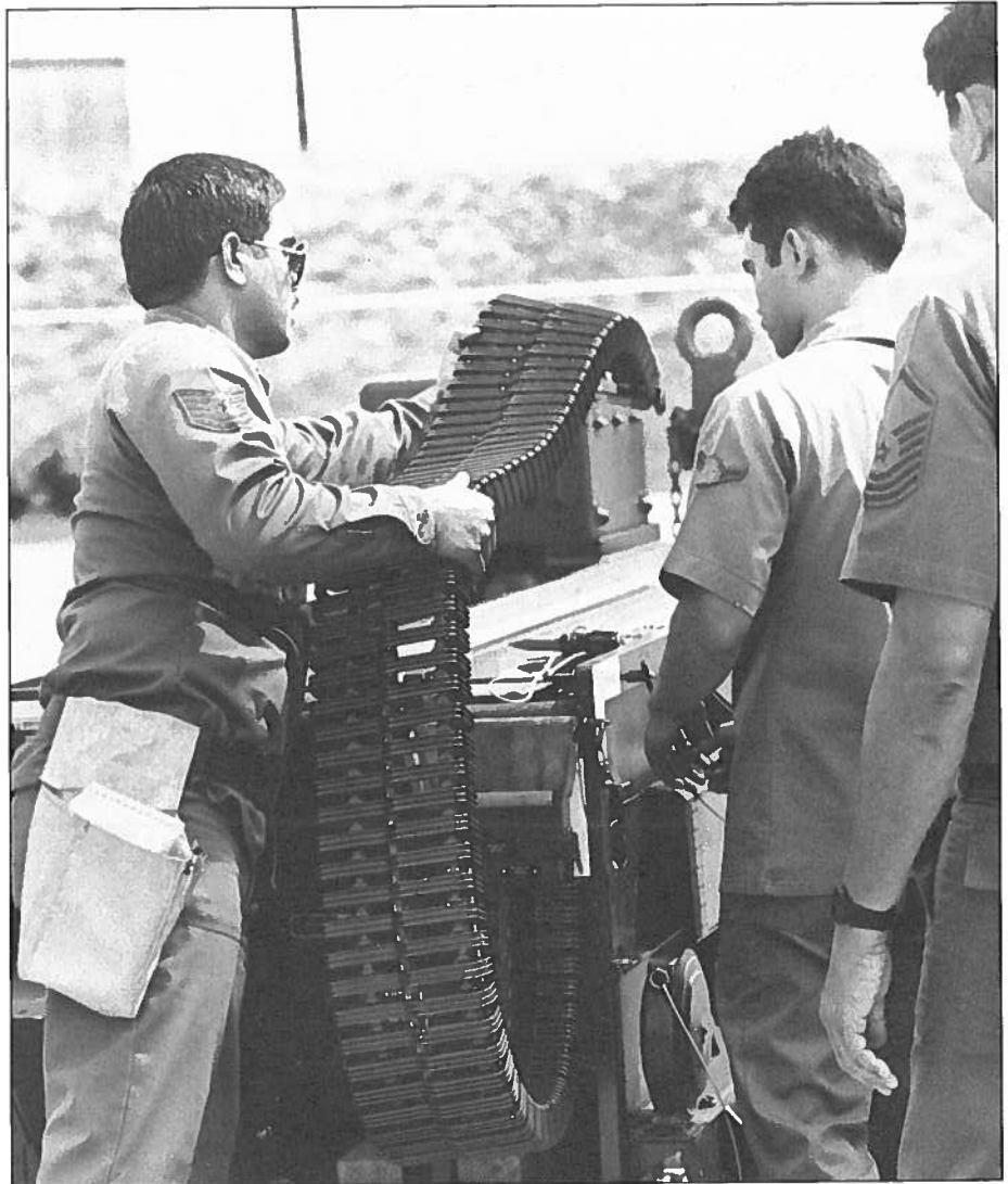
Munition technicians of the 154th Consolidated Maintenance Squadron load 20-mm rounds into ground servicing equipment prior to reloading an F-15 internal "Gatling" gun.
