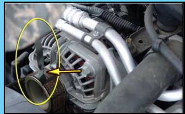
Airmen at the 375th Logistics Readiness Squadron, Scott Air Force Base, identified the pictured entanglement hazard with the ABU jackets lower arm vent draw cord. In this specific case, the hazard was discovered while checking transmission fluid.
