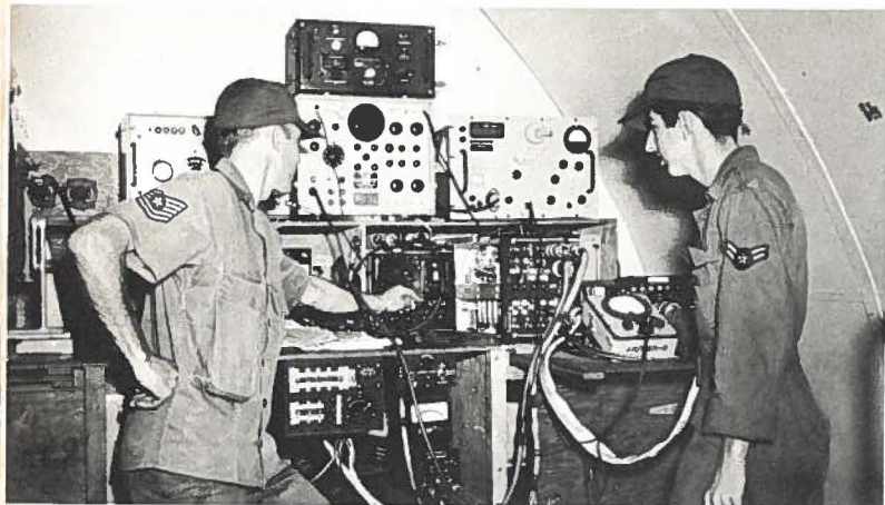
LIKE SO. TSgt Osborn D. Matlock and A2C David M. Rodrigues working on the AGPE 30, F-86E Fire Control System.
