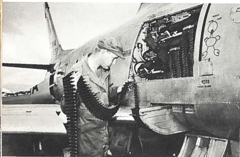
LETHAL PUNCH. A3C Wayne A. Hunter loading cal. .50 ammunition into a SABRE JET.
