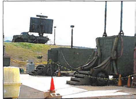
The new JTIDS module and Operations Module positioned below the TPS-75 radar
